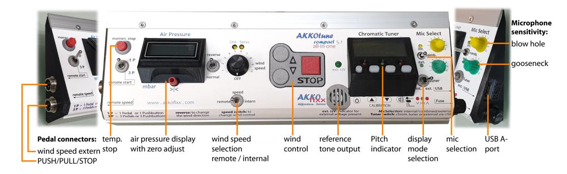
**As before:** Setting the air pressure, switching the wind direction, displaying the air pressure,
