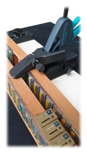
In order to blow both chambers of the same position or two reed blocks in parallel on a reed block, an insert with a slot is used; the stop is positioned so that the slot does not protrude beyond the sole of the reed block.
