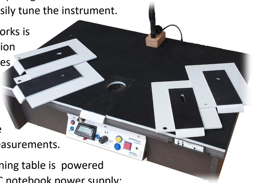
The needed air stream is generated by a special radial blower and may be switched instantly from PUSH to PULL. The blower speed is electronically controlled and the resulting air pressure is as well electronically measured and displayed on the front panel.
