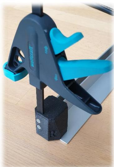
The arms with the hold-downs can be moved on the table top and are fixed with the star grip screws.
