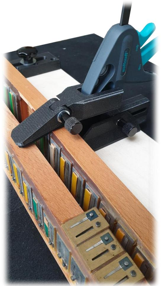
In order to blow both chambers of the same position or two reed blocks in parallel on a reed block, an insert with a slot is used; the stop is positioned so that the slot does not protrude beyond the sole of the reed block.
